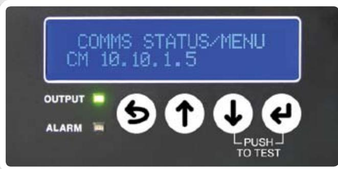
Displays IP address to verify network communication
