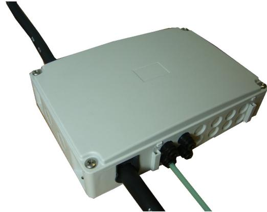
The Riser Box is designed for use within apartment blocks and mid/high rise office blocks. The unit houses a single integral splice tray, and allows fibres from an in-line or butt Blown Fibre tube cable to be spliced up to 12 customer drop cables. In cases where Blown Fibre tube cables are to be used for the customer drops, bulkhead tube connectors can be fitted to the unit.
